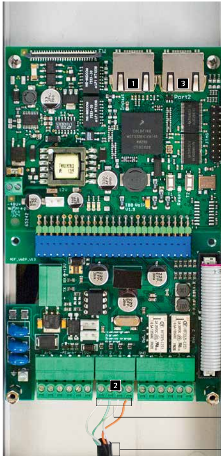
Ethernet connection according to EIA/TIA 568 A
